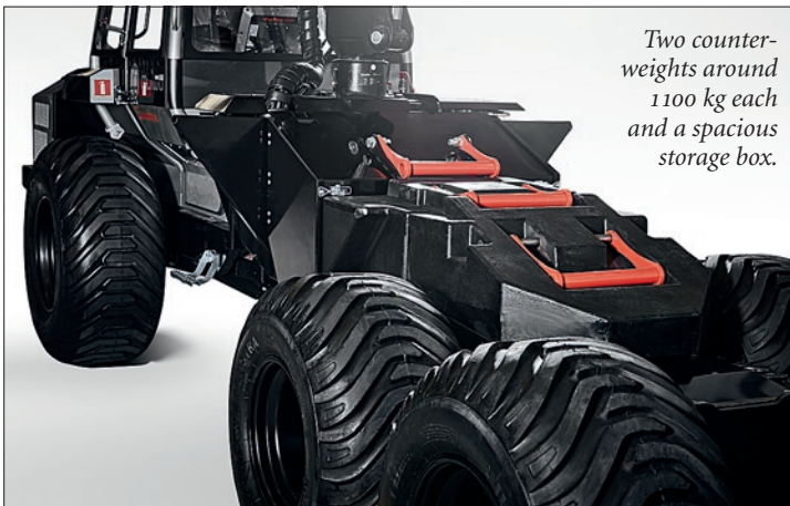
Conversion between harvester and forwarder takes about 20 minutes.
